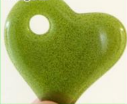
Image 2: Filled using only fine grain frit. Note the many small bubbles and foggy appearance.
