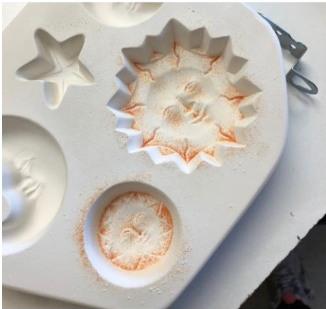
Sift powdered Cherry Red frit along the border and into the center of the face of the suns.
