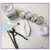
Prepare your mold well with suitable glass separator before adding glass. We recommend spray-on ZYP. Always wear a mask when using spray-on separators and/or powder frits.
