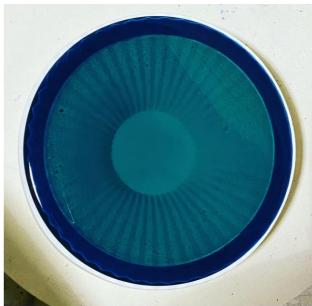
Allow the glass to cool. Treat the GM254 mold with ZYP and place the mold onto a level kiln shelf with a piece of kiln shelf paper underneath the mold so that the kiln shelf under the center hole of the mold is covered with the kiln shelf paper (see image above). Center the glass on the mold and fire the glass using this schedule:\*
