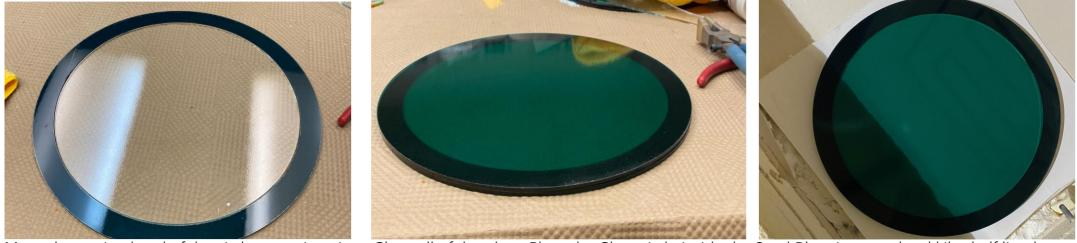
Move the cutting head of the circle cutter in a tiny bit (1/64") and cut a circle of COE 96 Standard Clear.
