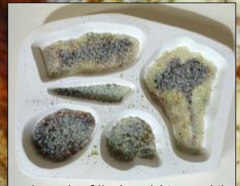
Place the filled mold into a kiln and Tack Fire using the following schedule.
