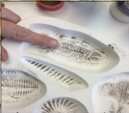
After your LF140 is primed and dry, sift F1 Black into each fossil and gently sweep it into the fine details with a finger. Take care to not move or remove any separator.
