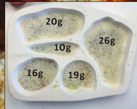
Add a layer of F3 Vanilla Cream to each mold until they're approximately 1/4" full of frit. If using fill weights, refer to the above image.
