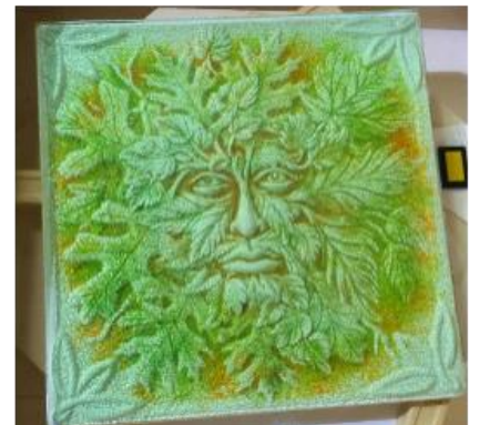
Once your frit is arranged as you like, top the mold with a 12" x 12" square of Citron followed by a 12" x 12" square of Standard Clear. Move the project onto 1" kiln posts on a level shelf in the kiln and fire to a Full Fuse using the suggested schedule in Table 1 or your own preferred Full Fuse with a bubble squeeze.
