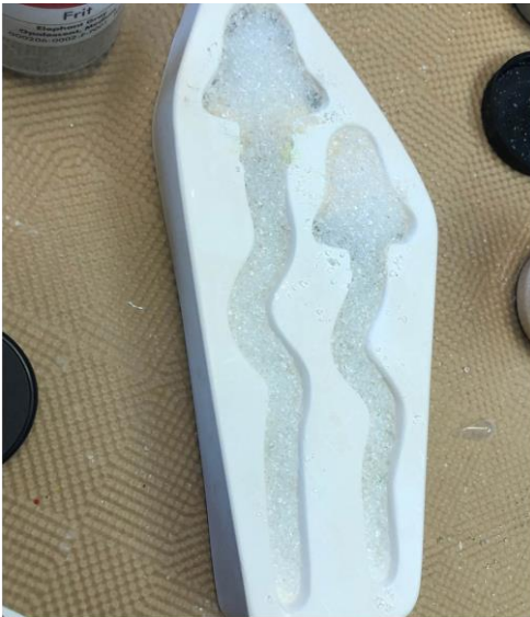
Fill the cavities with Medium Grain Clear frit until the tall mushroom cavity holds 62 grams frit and the short mushroom cavity holds 48 grams frit.
