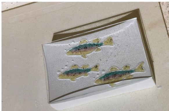
Cut a 5.75" x 3.5" rectangle out of 3m clear fuse-able sheet glass and place it on the mold in your kiln. Fire using the schedule found in table 1.
