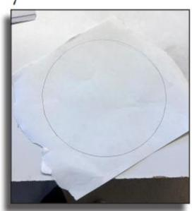
Trace a 9" diameter circle onto a sheet of Thin Fire Paper, and place it onto a kiln shelf.
