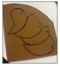
To transfer the pattern to the glass, first lay the glass over the pattern, then trace it with Sharpie. Make sure to include the number on each piece as well for an easier time placing them later.
