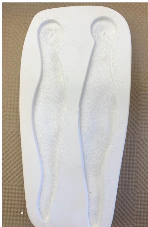
Fill both Gnome cavities with Clear frit. If you are weighing the mold fill it until the glass in the mold weighs 190 grams. Full fuse the mold using your favorite full fuse or the schedule we suggest in table 1.
