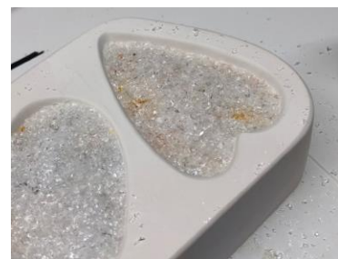
Slim Heart: Cherry Red trans, Orange trans, Marigold Opal stringers were used in the slim heart. Fire the mold to a full fuse. A suggested schedule can be found in Table 1.
