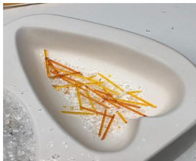
Break more Cherry Red, Black and White stringers and place the pieces in a random pattern over the Clear frit in the mold. Continue layering the stringers and Clear frit until you have filled the cavity with a last layer of Clear frit. The images shown above here were done in the wide heart. You can do the same technique in the slim heart see below for colors.
