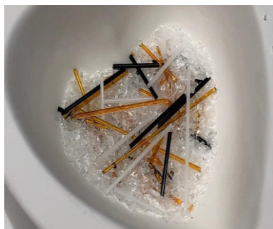
Break more Cherry Red, Black and White stringers and place the pieces in a random pattern over the Clear frit in the mold. Continue layering the stringers and Clear frit until you have filled the cavity with a last layer of Clear frit. The images shown above here were done in the wide heart. You can do the same technique in the slim heart see below for colors.
