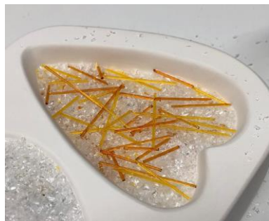
Slim Heart: Cherry Red trans, Orange trans, Marigold Opal stringers were used in the slim heart. Fire the mold to a full fuse. A suggested schedule can be found in Table 1.
