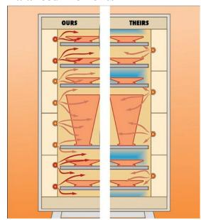
A large amount of the heat you lose in your kiln passes to through the lid and slab of your kiln. To compensate for this, Skutt directs more heat to these areas when they design the elements. The fact that we have twice the element grooves in our kilns gives us more design flexibility than some of our competitors.
