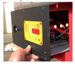
One of the most problematic components of kilns has traditionally been the relays. Mechanical relays have a limited life which is why Skutt has upgraded all Scarab Kilns with **Solid State Relays**. These relays or kept cool with a **fan mounted in the side** of the kiln (not necessary on the Mini Scarab because the Amps are so low).
