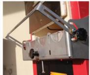
The Optional Secondary Point Rests, another unique design of Marcel Braun, are generally ordered on just about every Scarab that goes out of here. Flameworkers love its ability to hold long handles, preventing their work from popping up off the floor. Its well thought out design allows you to move the rest to almost any position you want. It not only moves in and out but also moves up and down. The scalloped edge ensures that your rods will stay in place. Do Not Forget To Order This Upgrade.
