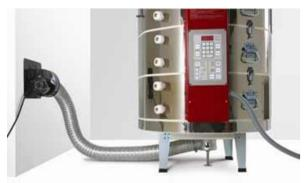
The EnviroVent 2 is what is known as a **Downdraft Vent**. Downdraft vents actively remove fumes from your kiln before they can enter the room and vent them outside keeping your studio free of smell. It works by using a wall mounted fan to draw a very small amount of air through holes drilled in the slab (floor). The amount of air drawn is determined by the number and size of the holes drilled. Holes are also drilled in the lid in a specific pattern designed
