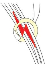
Skutt is one of the few brands that installs a **Current Sensor in every GlassMaster Kiln**. This allows you to read the **Amperage** of
