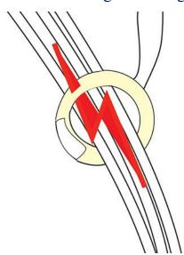
Skutt is one of the few brands that installs a **Current Sensor** in every GlassMaster Kiln. This allows you to read the **Amperage** of each section of the kiln as well as the **Voltage** and **Voltage Under Load**.
