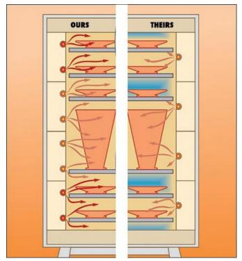
A large amount of the heat you lose in your kiln passes to through the lid and slab of your kiln. To compensate for this, Skutt directs more heat to these areas when they design the elements. The fact that we have twice the element grooves in our kilns gives us more design flexibility than some of our competitors.
