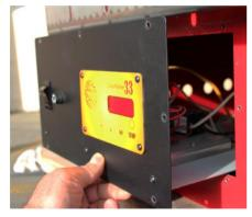
One of the most problematic components of kilns has traditionally been the relays. Mechanical relays have a limited life which is why Skutt has upgraded all Scarab Kilns with **Solid State Relays**. These relays or kept cool with a **fan mounted in the side** of the kiln (not necessary on the Mini and Micro Scarab because the Amps are so low).
