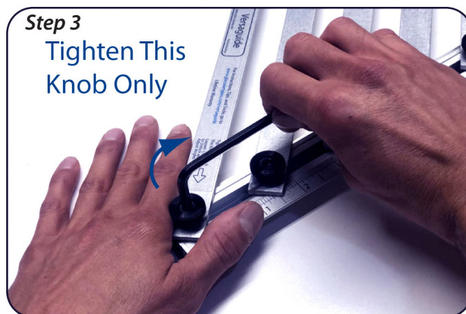
Hold firmly and use hex key to Re-tighten Lock Knob. DO NOT OVERTIGHTEN.
